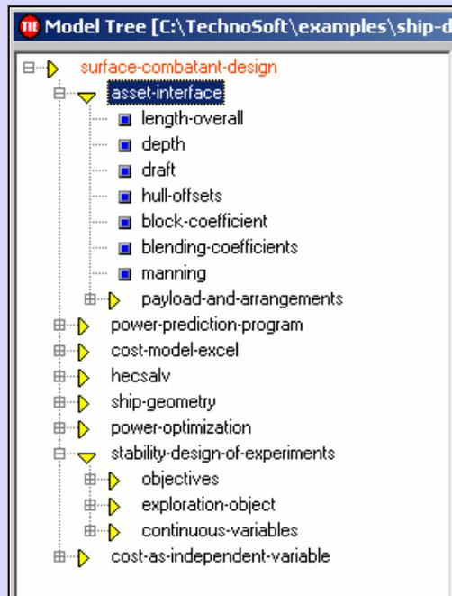
TechnoSoft is using its proven Adaptive Modeling Language (AML) to build a knowledge-based modeling environment for ship geometry, including the hull-form, internal compartments, and deck-house.
