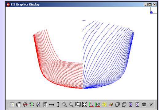
Surface Ship Evaluation Tool (ASSET). ASSET contains a wealth of naval architecture knowledge that is employed to make sure that the designer's inputs are consistent with the ship's purpose, and to make educated guesses for inputs which are not provided.
